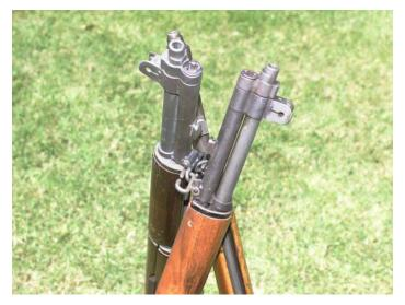
Figure A-18e.--Close Up of Stacking Swivels.
